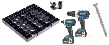
Attach the Silca Grates to joists using X6 countersunk head self-drilling screws per grate. 10G X 60 410 CSK SQ SELF DRILL WINGTEK.
