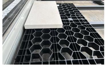
Where a free draining permeable surface and level entry through threshold is desired (no grout) a level structure can be built. For "permeable surface" and "level entry through threshold" a 5mm gap around each tile is required as detailed in E2/AS1 for permeability and level entry.
