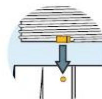
An unscrewing safety system preventing each element from detaching at the maximum height reached
