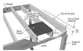
Install Silca System over typical timber joist deck structure or on adjustable pedestal over membrane.
